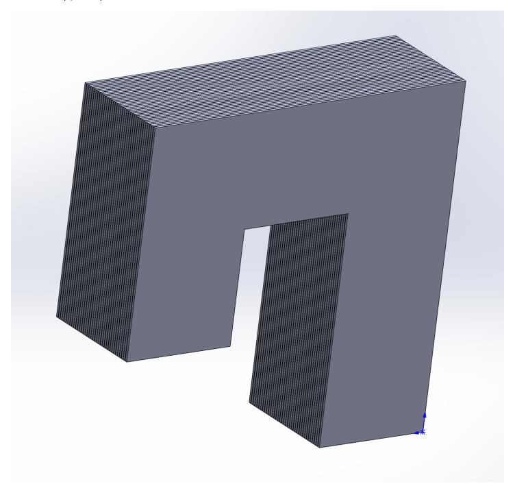
Pole (2 - 1/2 Pole Laminations butted together (no gap) to form 1 Pole [shades of gray for clairity]:
