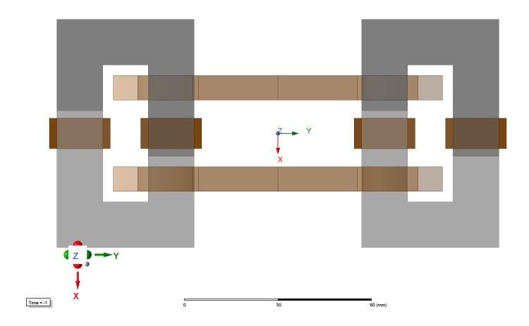
TFG\_Z04 Structure Top/Bottom View (Z) [Copper = Loop Coils, Lightish Copper = N/S Coils, Gray = Poles]:
