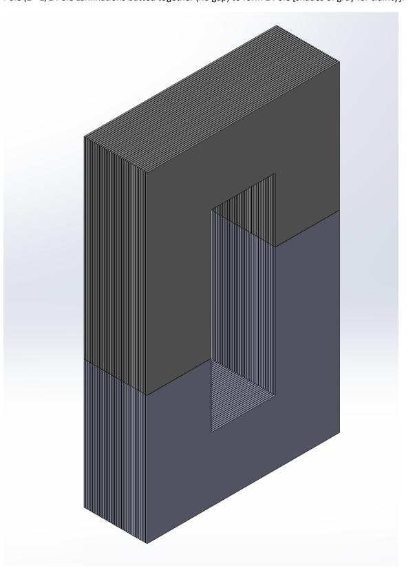
Lamination cut scheme to eliminate scrap [shades of blue for clairity]:
