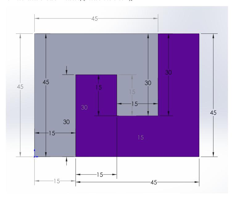
Lamination pattern for Laser/Waterjet cut [shades of blue for clairity]:
