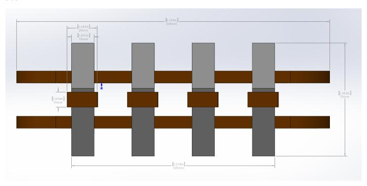
Laminated or solid electrical steel is used for the "U Pole" elements. Copper wire, stranded or solid makes up the N/S pole coils and the Loop coils.
