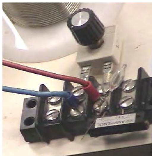
As there are very slight differences in the manufactured coils, each one is tuned to the exact transmitter frequency and a miniature neon is used to show when the tuning has been set correctly.
