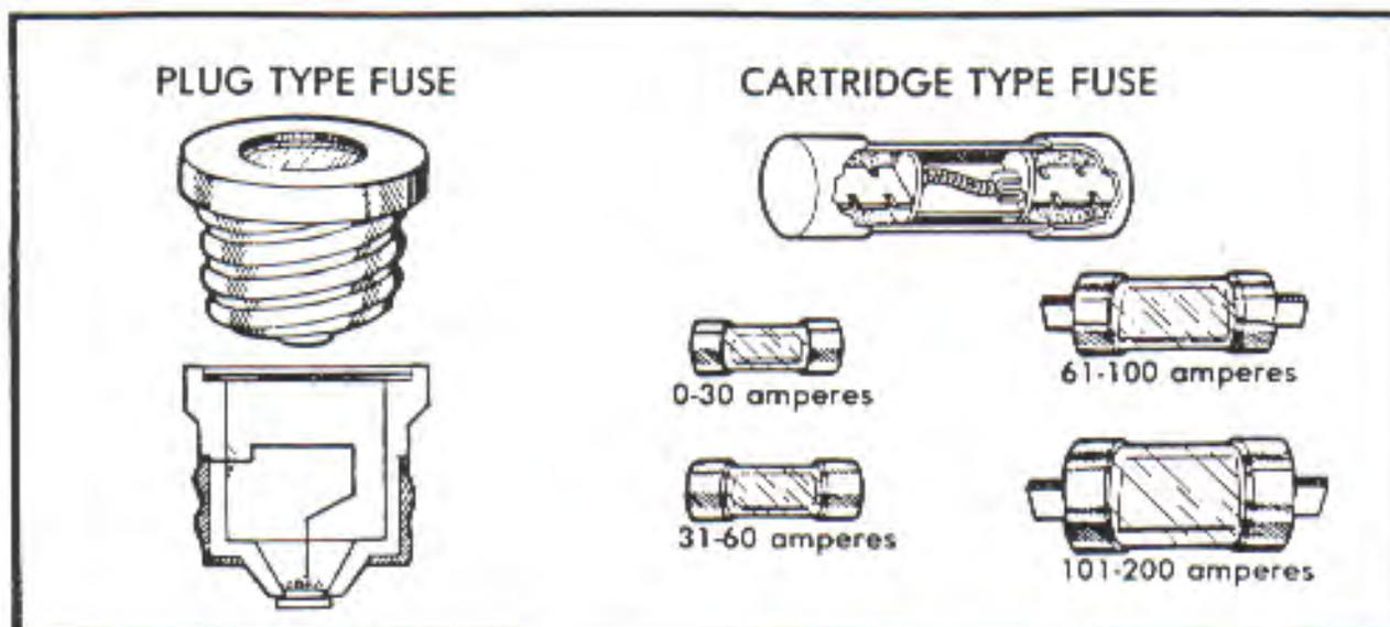
Fusetrons (time-delay fuses) are made to carry a temporary overload, such as the overload caused by the starting of an electric motor. The fuse, however, still provides protection for the circuit, and a short circuit will melt the fuse link. If a common fuse is used, the fuse link will melt every time an electric motor starts. The use of a larger ampere common fuse will prevent the "blow" resulting from the temporary overload, but will not provide protection for the motor or the circuit.
