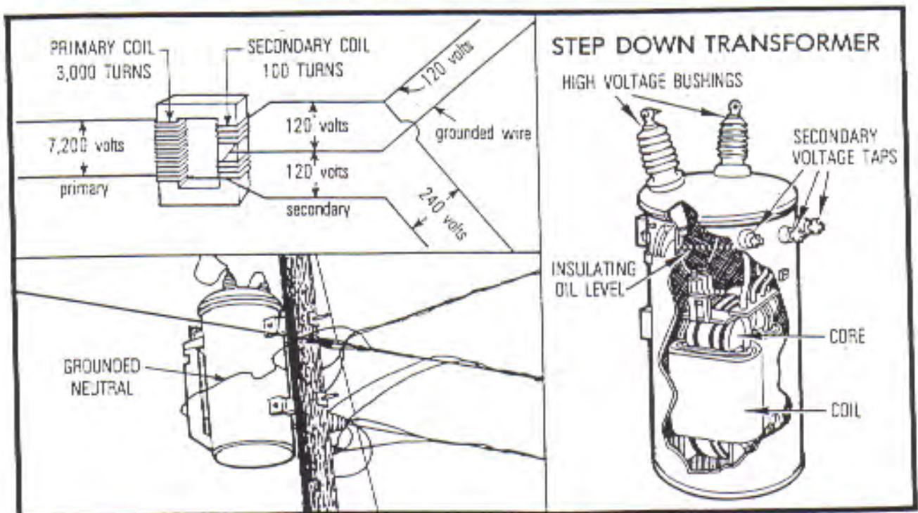
**Single Phase** - The most common type of electrical service or power available to consumers. One transformer is used between the distribution line and the meter. Usually three wires, two "hot" and one neutral, are installed to provide 120V and 240V single-phase service. Single-phase service may also be supplied with three-phase service.
