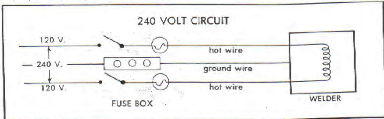
The voltage on a 240V circuit is measured by fastening a lead on the voltmeter to each of the hot wires. Voltage between either hot terminal and the neutral bar will be one-half of the voltage between the two hot wires. The number of amperes flowing can be measured by clamping an ammeter around either of the hot wires.
