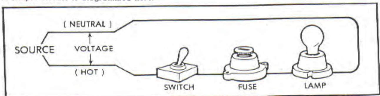
A circuit includes a "hot" wire (red or black) carrying current from the source through a switch, circuit protector (fuse or circuit breaker), and an appliance. The neutral wire (white) conducts the current from the appliance to the source (ground).
