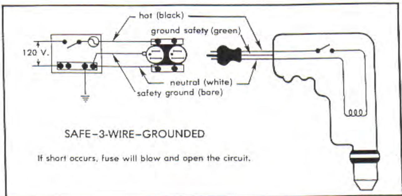
Using grounded receptacles and a safety-ground on all circuits will allow the safety-grounding of appliances when they are plugged into the outlet. An adapter must be used to properly ground appliances connected to receptacles not safety-grounded. If an adapter is used, the green pigtail wire must be connected to a known ground to give protection from electrical shock should a short occur.
