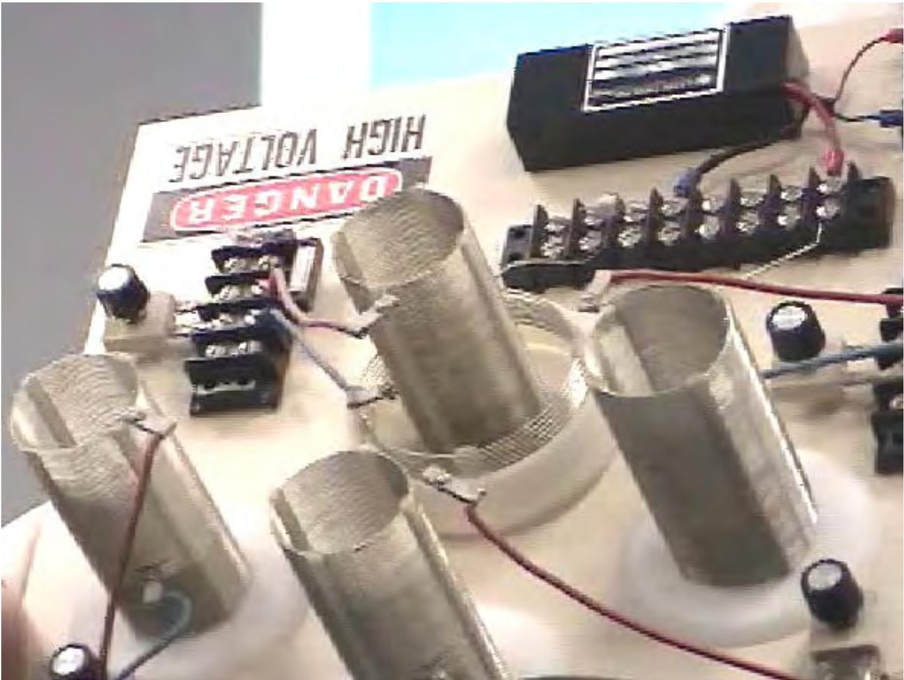
The secondary coils are constructed using Barker & Williamson's normal method of using slotted strips to hold the tinned, solid copper wire turns in place.
