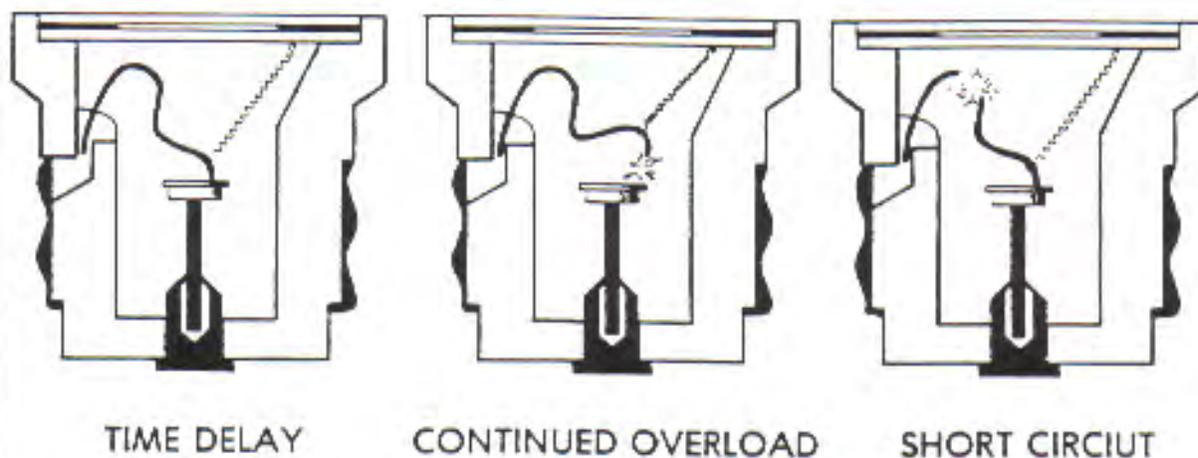
Fustats, nontamperable fuses of the time-delay type, have a different size base and require a special adapter that is screwed into the standard fuse socket. After the adapter is installed, it cannot be removed. For example, the installation of a 15-ampere adapter allows only the use of 15-ampere or smaller fuses.
