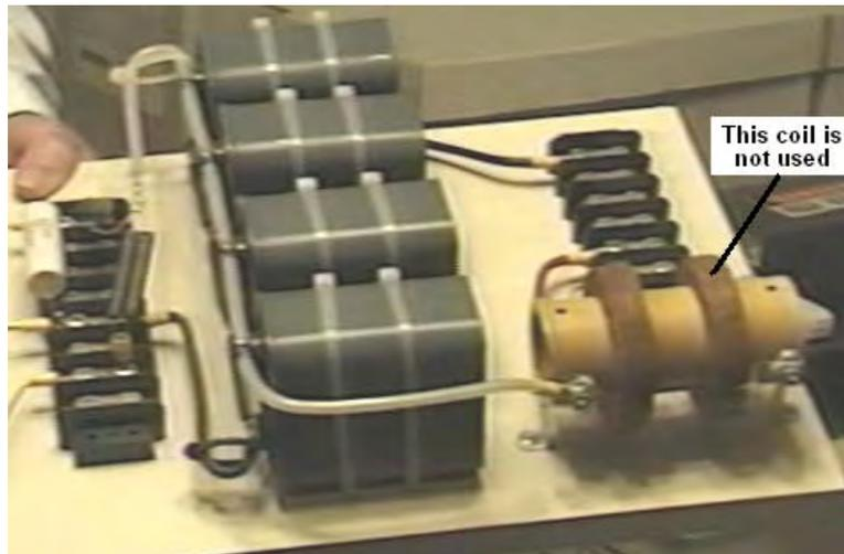
The output current flows through the left hand winding on the brown cylindrical former, and when the photograph was taken, the right-hand winding was no longer in use. Previously, it had been used to provide charging power to the battery by rectifying the electrical power in the coil, caused by the fluctuating magnetic field caused by the pulsing current flowing through the left hand winding, as shown here:
