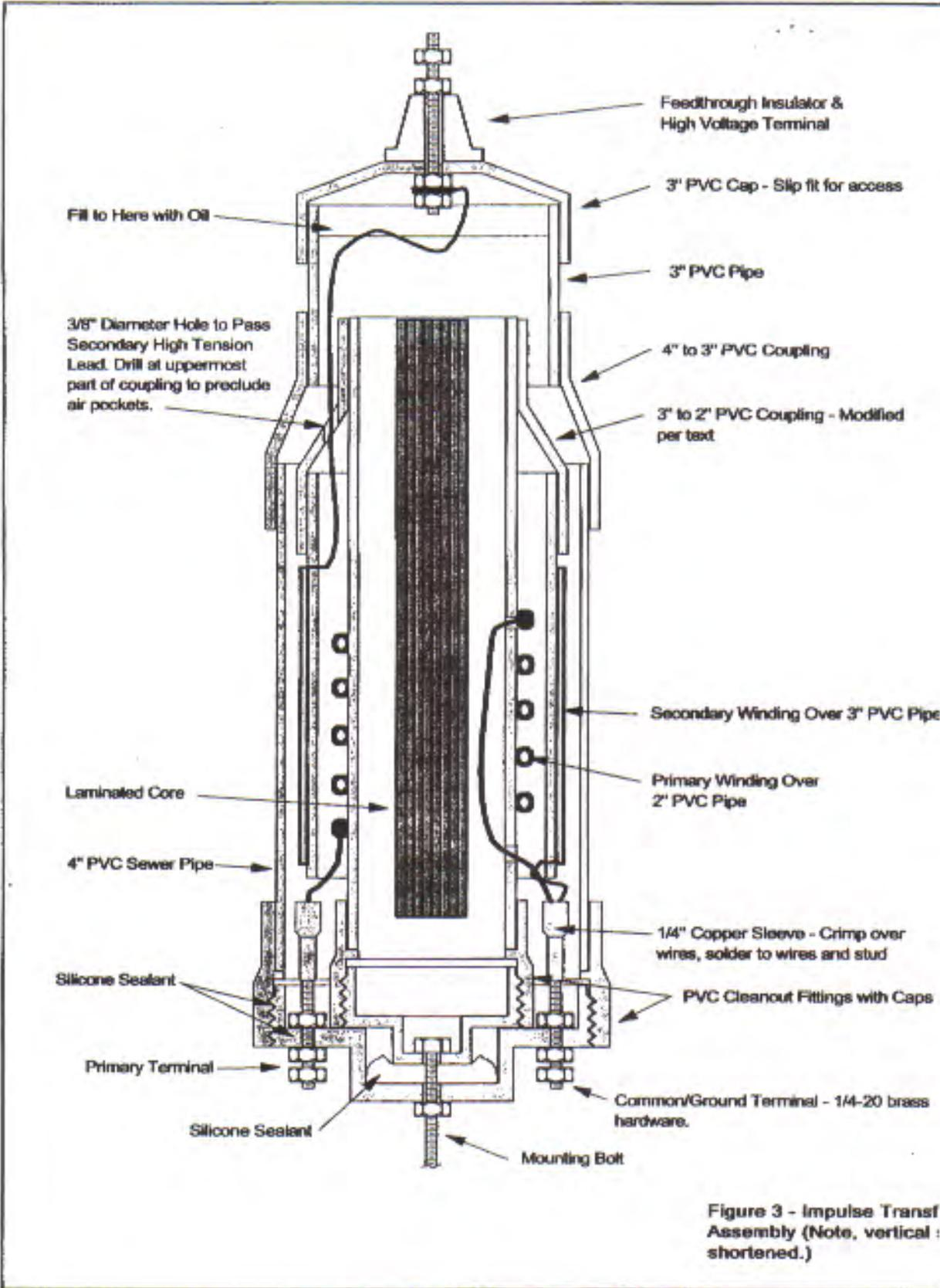
**Figure 3 - Impulse Transf Assembly (Note, vertical : shortened.)**
