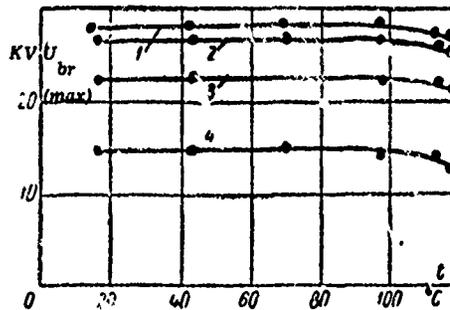
Fig. 51. Dependence of  $U_{br}$  of carefully purified transformer oil on temperature for various pressures over the liquid. 1-  $p = 750$  mm hg; 2-  $p = 500$  mm hg; 3-  $p = 250$  mm hg; 4-  $p = 10$  mm hg.
