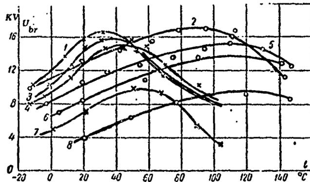
Fig. 62. Dependence of  $U_{br}$  of xylene and transformer oil on temperature for various frequencies. 1,3,4,5 xylene; 2,5,6,8 - transformer oil; 1 and 2 -  $f=4 \times 10^5$  hz; 3 and 5 -  $f=8.6 \times 10^5$  hz; 4 and 6 -  $f=2.4$  mhz; 7 and 8 -  $f=12$  mhz.
