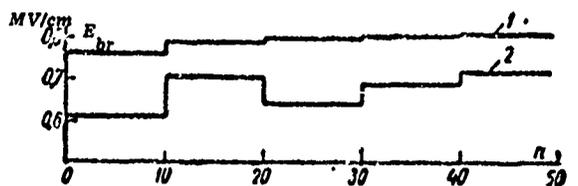
Fig. 64. Effect of electrode material on  $E_{br}$  for hexane. 1- electrodes of chromium; 2- electrodes of silver.
