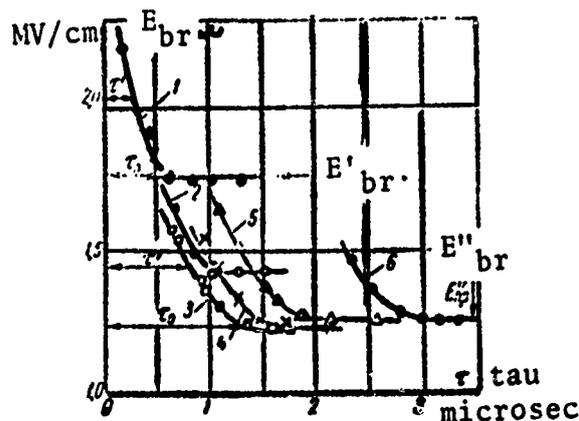
Fig. 41. The change in  $E_{br}$  of N-hexane for various square pulse durations and inter-electrodes distances 1. 1- 1 = 33 microns; 2- 1 = 41 microns; 3- 1 = 47 microns; 4- 1 = 54 microns; 5- 1 = 61 microns; 6- 1 = 68.5 microns.
