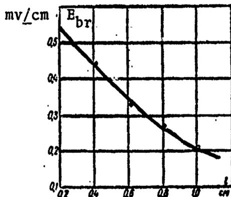
Fig. 27. The Dependence of  $E_{br}$  of sovtol on inter-electrode distance for pulse voltage (according to Panov and Mravyan)
