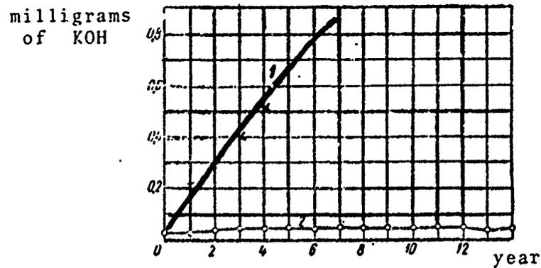
Fig. 80. The acidity of turbine oil as a function of time. 1 - oil without antioxidant; 2 - oil with anti-oxidant.
