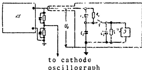
Fig. 92. System for measuring of currents in the case of short rectangular pulses.
