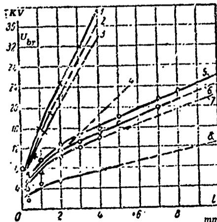
Fig. 61. Dependence of  $U_{br}$  of xylene on interelectrode distance for various frequencies. 1- sphere-sphere,  $f=4 \times 10^5$  hz; 2- same, but  $f=8.6 \times 10^5$  hz; 3- same, but  $f=2.4$  mhz; 4- same, but  $f=12$  mhz; 5- point-sphere,  $f=4 \times 10^5$  hz; 6- same, but  $f=8.6 \times 10^5$  hz; 7- same, but  $f=2.4$  mhz; 8- same, but  $f=12$  mhz.
