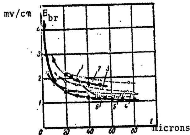
Fig. 25. The dependence of  $E_{br}$  On Spark Gap Widths For Various Hydrocarbon Liquids
