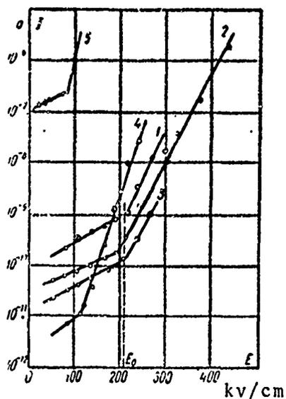
Fig. 87. Current as a function of the voltage of field applied at various temperatures  $t$ . 1-highly purified xylene,  $t=80^\circ\text{C}$ ; 2-the same at  $t=0^\circ\text{C}$ ; 3-the same at  $t=-20^\circ\text{C}$ ; 4-purified heptane; 5-purified chlorobenzene
