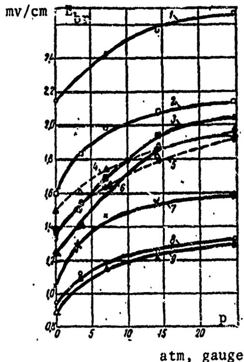
Fig. 21. The dependence of  $E_{br}$  of degassed liquids on external pressure. 1-hydrocarbon substituted with four chlorines; 2-N-decane; 3-toluene; 4-N-heptane; 5-N-hexane; 6-benzine; 7-chlorobenzine; 8-ethyl alcohol; 9-methyl alcohol
