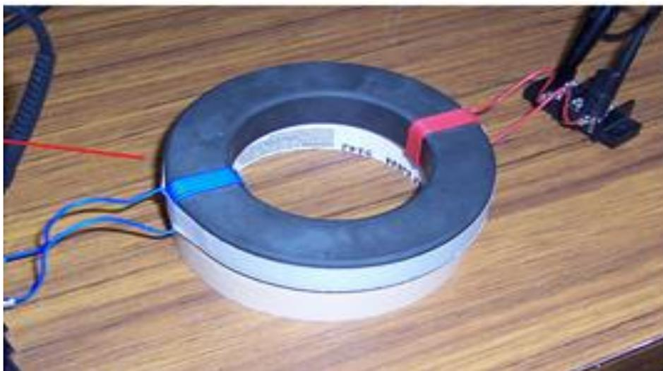
**Figure 2. Magnetic delay transformer**
